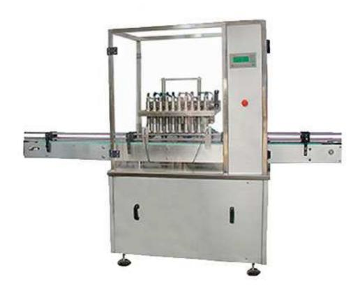
R-XP/A Bottle Air washing machine with the function for removing the dust and dirt that have settled during shipment transfer. The inline nozzles deliver short bursts of clean air into the bottles to removing the static charge on the bottle inner-walls and suspending the contaminants in midair. These contaminants are simultaneously vacuumed out by these nozzles, then the pre-washed bottles can be move into the next filling station.
