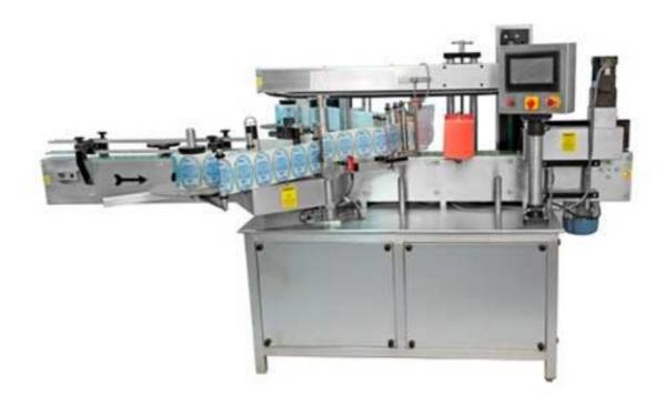
This double side flat bottle sticker labeling machine offers superior production and quality labeling of bottles. The flat bottle labeler achieve double side sticker stamping on bottles of different materials, diameter and height. This double side bottle sticker labeling machine achieves custom labeling rate for bottles per minute based on the type of model. The bottles are in-feed using feed screw and these pass to conveyor that holds the products from top.
