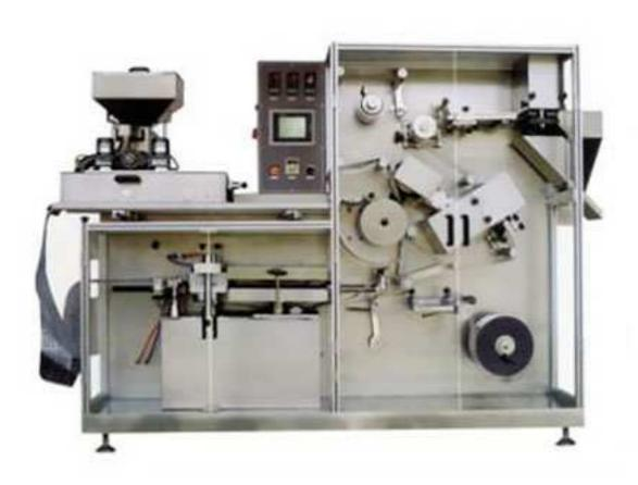
This roller type Aluminium-plastic Blister Packing Machine is used for packing different sizes and shapes of tablet, capsule, pill, candy and other solid granule type product. It can be used in the pharmaceutical, foodstuff and chemical industry.
