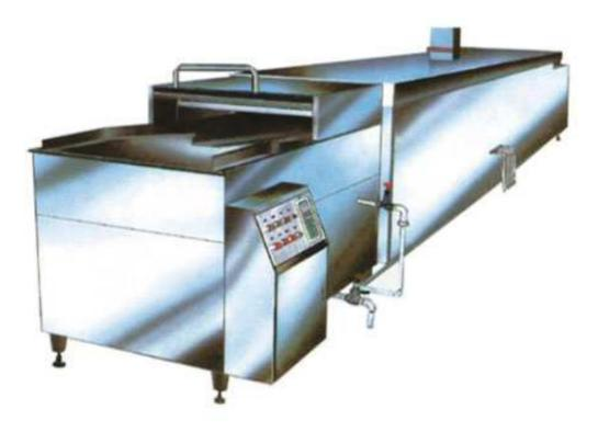
This boil bottle sterilizing machine is mainly used for boil sterilization for ampoules and oral liquid bottles, and it conforms to GMP standards. Bottles are first washed by preheating sprayer, and then they will be automatically conveyed to water channel for boil sterilization whose effects can be better if the ultrasonic waves are used together. Meanwhile, impurities of bottles like dust, sand can also be removed.
