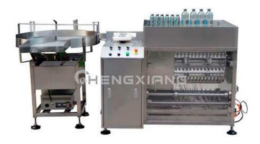
This machine is mainly suitable for 20-500ml shoulder all kinds of round bottles or special-shaped bottle to bottle cleaning inside and outside, by two in water (tap water and ionized water, no oil compressed air) alternate irrigation. The bottle meet production process requirements, and the initial dry bottle, etc. This machine can be wired or standalone use. This equipment is fully in line with the new version of GMP requirements
