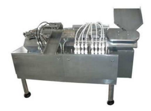
Apply sample trial test and small batch production in pharmaceutical industry, ampoule filling and sealing in the condition of sterile.
