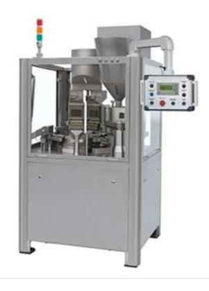
NJP-2000, 2500 series automatic capsule filling machine based on old NJP-2000 series, designed total enclosure turning table for easy cleaning, single movement for both upper and lower segments with two-lip seal provide a much better sealing performance, a combined air blowing & suction function on segment cleaning station ensures cleaning efficiency on high speed, dust-preventing rubber block on capsule discharge station.
