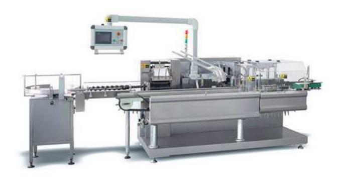
This machine is suitable for automatic feeding bottle (round, square bottle) into carton (either for blister or bottle). Online bottle unscramble and feeding, leaflet fold (1-4folds) and feeding, leaflet detecting, canton opening and forming, products and leaflet pushing into carton, printing batch number, sealing carton with tuck-In or hot melt glue device Automatically reject lacking of leaflet or product and finished product out.
