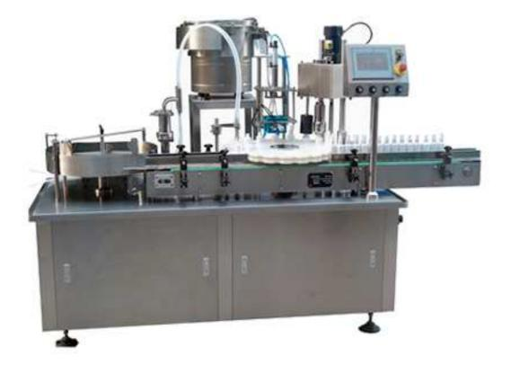
This glass dropper bottle filling and capping machine includes the turn table feeding bottle, automatic filling, automatic feeding sprayer pumps (glass dropper), capping, labelling and bottle collection table.
