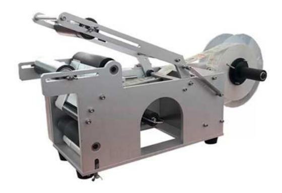
This semi automatic flat bottle labeling machine is a tabular semi-automatic machine with motor and touch control via limit switches and small size, suitable for matching with vertical filling and packaging machines and for printing production dates and batches of industrial foods, beverages, pharmaceuticals, etc.
