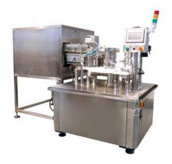
DLF-2 is new generation liquid filler and capper which can complete the process of filling, cap feeding and capping on one machine FOR Diagnostic Reagent tube. It is easy to operate and adjustment. The advantage design could complete the tube sorting and feeding, cap sorting and feeding automatically. DLF-2 can fill different kinds of liquid in pharmaceutical and chemical industry with high precision.
