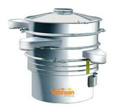
Powder sieving machine is designed as a high-precision screening machinery. Vibrating screen is composed of vertical motor, and eccentric weight installed at two ends. We can produce horizontal, vertical, inclined motions by adjusting the upper and lower eccentric weight. Diameter can be ranged from 400mm to 2000mm, with single or multiple screening decks (1-5 layers). Material can be divided into all carton steel, contact part stainless steel and all stainless steel.
