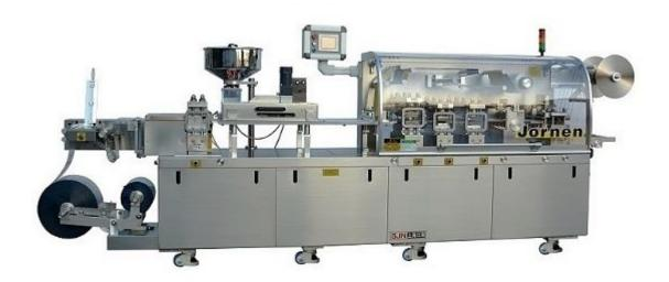
Blister Machine DPP260Ki-2 is classified electromechanical machines fully automated continuous horizontal type intended for the vacuum packaging of medical preparations (tablets, capsules).
