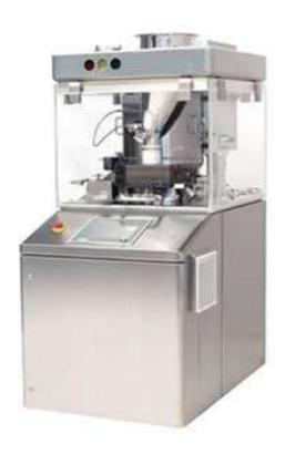
Rotary tablet press machine GTI-R series is is continuous automatic tablet press machine for pressing granular raw materials into tablets. It is mainly used in pharmaceutical, chemistry, foodstuff, and electronic industries and suitable for making large size tablets. It can provide double-layer tablets and effervescent tablets solutions, providing users with a variety of tablet pressing options.
