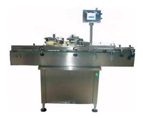
DLTB-A is economical, self contained, easy to operate, equipped with auto teach programming touch screen. Built in microchip storing different job setting makes fast and easy changeover.
