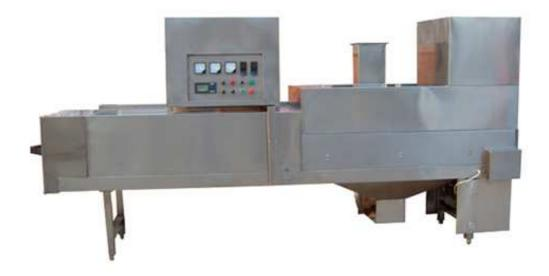
This machine is applied to dry, sterilize various glass bottles, such as oral liquor, clinical bottle and dropping bottle, and transfer by web sling (or chain). The speed of the web sling is adjustable. Heat with far infrared quartz tube to raise the temperature quickly with high efficiency. The temperature is shown on the temperature controller and may be automatically set, controlled and recorded.
