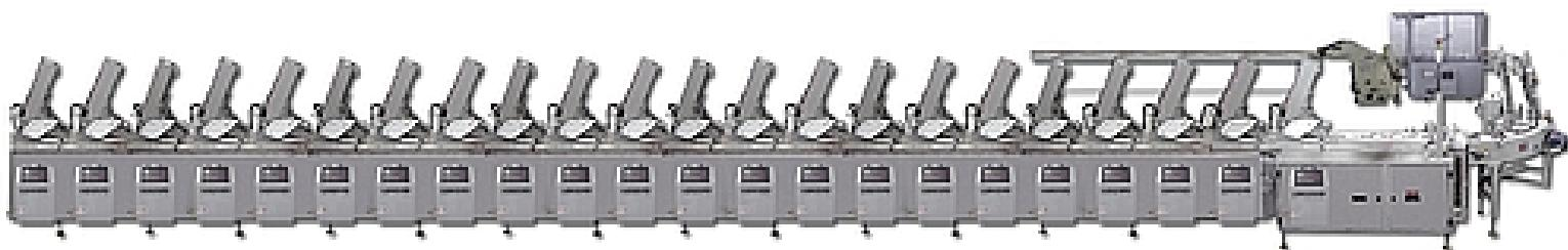
Provide massive labour savings and collation quality assurance by installing a custom selective collator that discharges directly into a high speed folder gluer. Design/build a (24) station custom selective collator that feeds, collates, shingles, stacks and transfers stacks of carton blanks into the infeed of a folder gluer. Line must allow for speed fluctuations of folder/gluer by having an inline buffer/shingled system.
