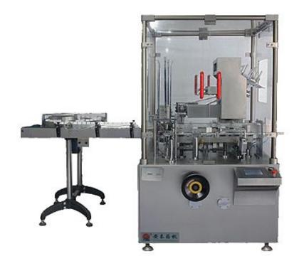
This machine is suitable for cardboard case packaging of blister package for blister package and similar package. It consists of direction folding (1-4 folds) and feeding equipment, cardboard case forming and feeding, batch number printing, sealing of case tongues at both ends etc. The whole encasing process is finished automatically. It can be added hot-glue machine.
