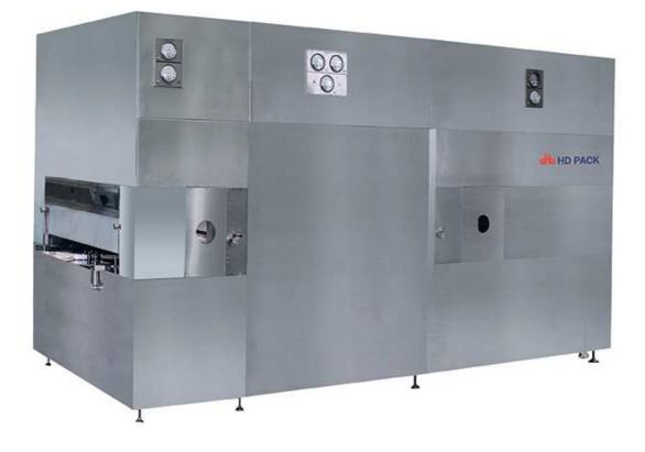
HD-SDT Series are designed to sterilize and dehydrogenate ampoules or glass vials by a laminar flow of hot air at up to 350 degrees. It is constructed with 3 parts, preheating zone, heating zone and cooling zones. After clean vials are sent to the sterilizing and Drying Tunnel automatically, they will be completely sterilized and dried in the airtight tunnel of laminar flows.
