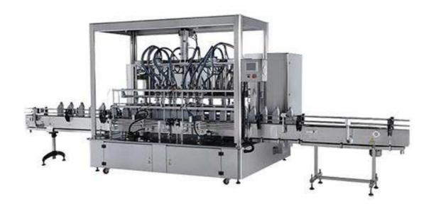
C serials are spiral pump filling machine with fast change-over design. Its exceedingly flexible performance is capable of filling think and semi-viscous liquid. This filler is most ideal for filling lubricant oil.
