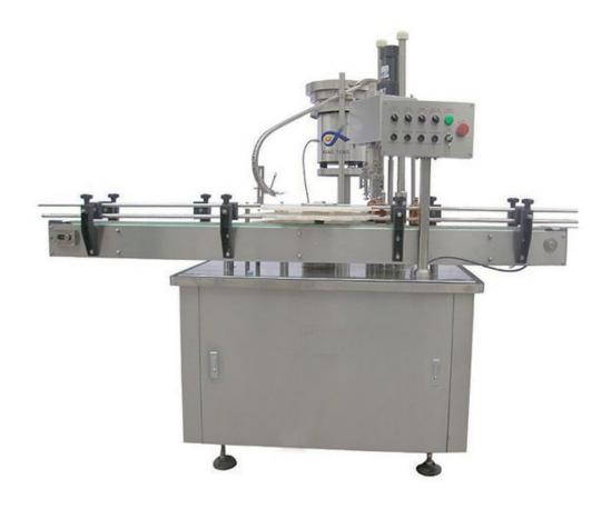
It used for cap putting, screwing and rolling and pressing work of unmoral shape bottles with different materials and specifications. Screw tops, theft-proofing caps, press-in caps and other cap types are applicable. It is convenient to adjust pressure with the adopting of constant torque capscrewing head. Structure is reasonable and compact, so this machine is convenient to be matched to other machines. Dust guard is selectable.
