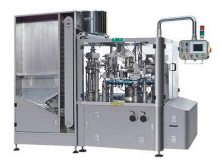
Automatic tube filling and sealing machine used for plastic, aluminum, laminate tube. It is one of main latest products of our company. It is full automatic. This machine can be used for filling cream and liquid materials.
