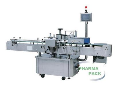
Equipped with advanced servo-motor driven labeling head, repeatable labeling accuracy is 0.5 mm. Dual rollers to ensure label dispensing accurately, compact design for easy changeover of labels.
