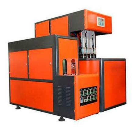
Semi automatic blow molding machine is suitable for producing PET plastic containers and bottles in all shapes. It is widely used to produce the carbonated bottle, mineral water, pesticide bottle oil bottle cosmetics, wide-mouth bottle and hot fill bottle etc.
