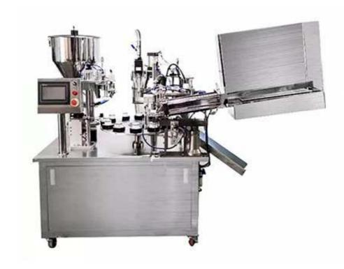
This machine adopts a digital adjustment system for filling volume, which can directly adjust the filling volume on the touch screen. The filling volume adjustment is convenient, accurate, stable and reliable.
