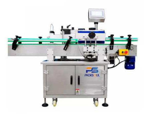
Sticker labeling machine is able to label different containers of different materials (plastic, glass, metal etc.) and different shapes (round, oval, rectangle, flat, irregular etc.). PSV-S101 serious labeling machine is used for single side labeling or full-circle on round surface of different shape containers.
