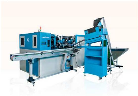
This is a new generation of fully automatic and versatile machine for mass production of PET large volume bottles, oval bottles, flat bottles and jars with volumes up to approximately 6000ml. Ideally suitable for applications where stringent quality requirements have to be met. Suitable for clean lotion, edible oil, detergent, pickle food, etc.
