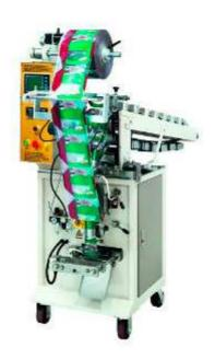
Model No. GTL-200-VLCY (Irregular Solids) Bucket Conveyor Feeding
