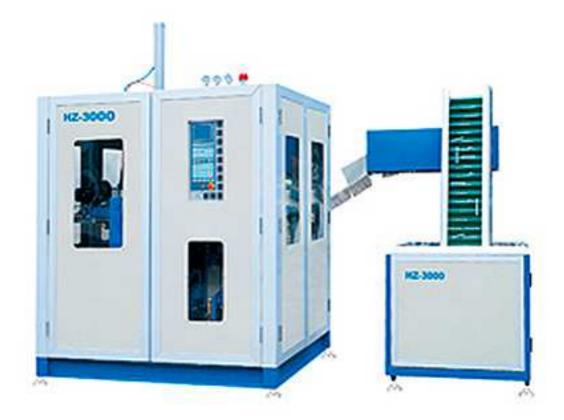
HZ-3000 Blow Molding Machine Suitable for CO2 bottle, mineral water bottle, pharmaceutical bottle, oil bottle, cosmetic bottle, hot filling bottle
