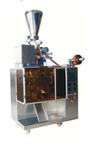
D-429CO series machinery is for the particles, powder, sheet and other materials to achieve automatic packaging design of the two-row roller packaging machinery. The machine can be made to carry a long strip of paste.
