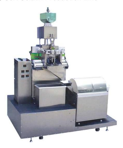
The new YWJ100 soft gelatin encapsulation machine (for laboratory) is elaborately designed on the base of bulk production type of 152 and 182 and according to the requirements of GMP standard. It is a simple and efficient laboratory machine, 220V power supply is used by the whole equipment. It is mainly for R&D or small batch production of gelatin capsule products in laboratories or pharmaceutical researching institutes.
