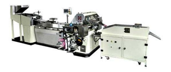
This candy roll wrapper machine apply to wrap candy with coincident shape, one set with several pieces cylindrical candy. Candy wrapped shape includes flat end and double twist.
