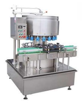
The machine is suitable for different bottles of ration liquid filling, Such as: no- carbon dioxide gas wine, beverages, condiments, liquid medicine and other liquid glass bottles.
