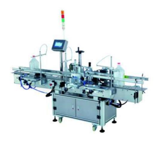
Applies to food, grain and oil and other industries, design for the need of fast automatic labeling on square and round material.
