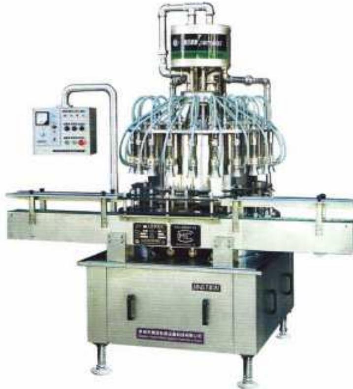
This machine is negative pressure filler, no work no filling bottles and broken bottles, filling accurate measurement, cup-type measurement (adjustable), automatic control valve pneumatic membrane surface, only need to replace some of the other parts, that is, Suitable for 80-1000ml automatic filling all kinds of packaging containers.
