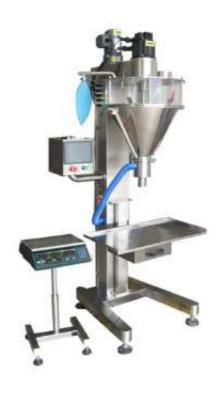
Semi-Automatic Powder Filling Weighing Packing Machine can also work as semiautomatic Detergent Powder or Soy Milk Powder Packing Machine.
