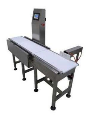
The checkweigher is suitable for testing the weight of a small single item whether is qualified or not, and it is widely used in electronic, food, pharmaceutical, beverage, health-care, chemical industry etc. F or example, it can be used in food industry to check the weight of flavour, cake, hams, instant noodles, frozen food, food additives, preservative etc.
