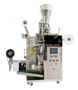
Tea Pouch Packing Machine is suitable for one-time packing of small particles such as tea, medicinal tea, health tea, etc. Equipped with Weighing Machine and material conveying system, tea packaging can be completed. Such tea Sachets Packing Machine is small in size, fast in packing speed and cheap in price.
