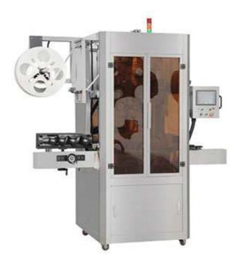
Sleeving labeling machine adopts PLC programmable controller, imported servo motor, servo driver, frequency converter and transducer;
