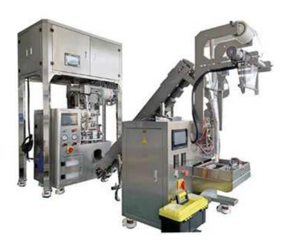
The main feature of the angle inner and uter bag packing machine is the one-time molding of the inner and outer bags to avoid the direct contact material by workers and improve efficiency. The inner bag is filter cotton paper, which can be automatically wired and labeled, and the outer bag is compound paper.
