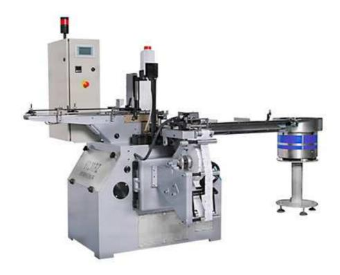
The full-automatic double-cube sugar wrapping machine is designed to convey the products to the customers in hygienic conditions and produced using high technology. The flexibility of adjustment is proper wrapping in different sizes by changing patterns.
