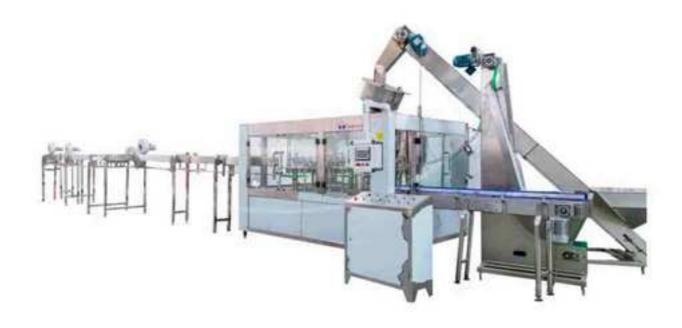
Our newly designed CGF serious monoblack water filling machine is designed for plastic bottle filling, it can suit for PET bottle size between 150ml to 2000ml, can customized to maximum of 3000ml. Genus design of capping design makes different screw cap change into one simple easy torch. On machine surface is only leaving 3 points of bearing support point which makes drainage so easy and without any dirt stain.
