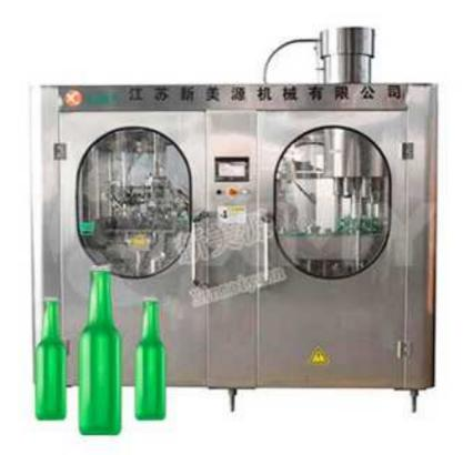
Carbonated soft drink/water/beverage filling machine is specially designed for small to medium scale production of both still and carbonated soft drinks such as coca cola, spirit, soda water, etc in PET bottles ranging in size from 0.2 to 2 liters, integrating rising, filling and capping into one.
