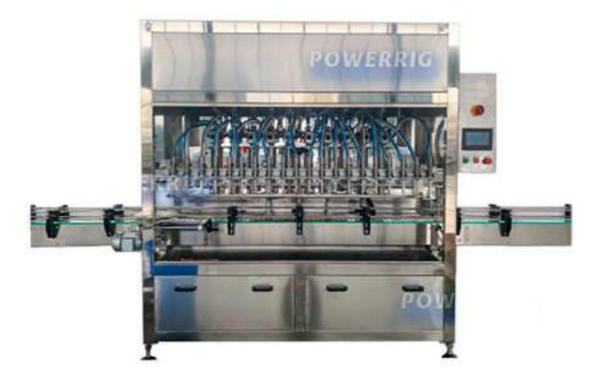
This Automatic Bottle Filling Machine adopts serve ball-screw system to drive the piston cylinder. It's widely used in Food, Chemical, Medical, Cosmetics, Agrochemical industry, applicable for filling liquid, especially for high viscosity material and foamy liquid, such as: Oil, Sauce, Ketchup, Syrup, Detergent, Honey, Shampoo, Lotion, Lubricant oil, etc.
