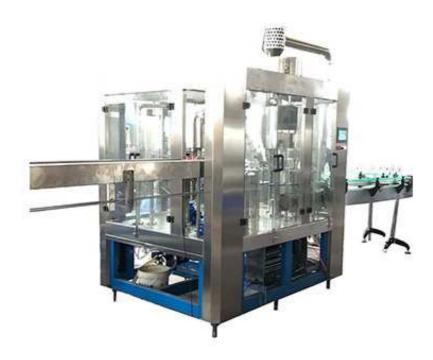
Automatic machine for bottle washing filling and capping, with 18 washing chucks, 18 filling valve and 6 capping heads, production capacity for 500ml mineral water is 4000-6000 bottles per hour. The available bottle sizes for this machine are 300ml – 2000ml.
