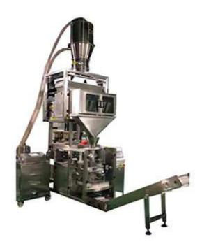
It cans fully automatic process including weighing, filling, film-pulling, making bags, printing, bag sealing and cutting. Machine including HDP-420 PE film packing machine, 4 heads linear weigher, weigher dust cover, vacuum feeder system, finished product conveyor, dater printer.
