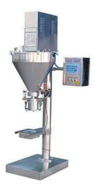
FC bag-clamping weighing packing machine is suitable for powder, granule and particles filling. The machine adopts two-speed screw feeding speed, pneumatic clamping automatic bag, electronic weighing filling. FC bag-clamping powder weighing packing machine can achieve highprecision automatic quantitative, automatic filling.
