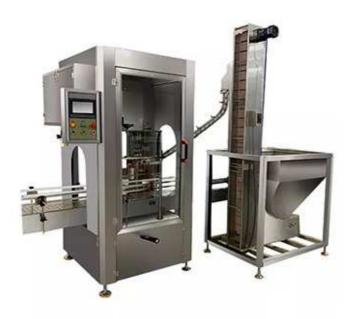
The machine adopts linear bottle feeding, PLC program control, double cylinder bottle positioning, can clear up and drop the cap automatically. Single-head machine in the double action lifting cylinder to grasp the cover firstly, then screw cap. The screw cap adopts the air expansion type catch cap, and is equipped with clutch device, the screw cap will not damage the bottle cap, the machine is suitable for the screw cap of the barrel with large diameter.
