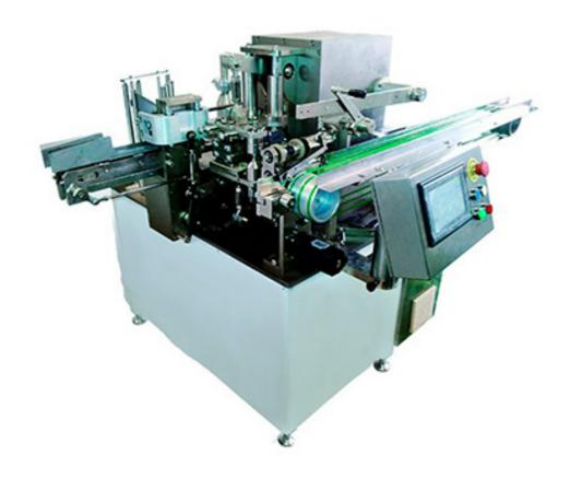
The Model DXDW120 is an automatic envelope packing machine. DXDW120 puts teabag into envelope packing solutions. Our company respond to market demand for envelope packing machine which is connected to the other teabag packing machine, the DXDW120 offers teabag sealed into envelope to suit customer's demands. The individual envelope offers a way to improve the filter bag's moisture proof refreshment. The printing of envelope has been designed to meet the requirements of our customers
