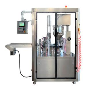
This machine is designed for coffee powder products (or other types of powder products such as cocoa powder, milk powder, etc.) to be filled and sealed in empty plastic nespresso capsules. It is characterized by compact structure, high degree of automation, easy to use, stable performance, simple maintenance, high production efficiency, 24 hours continuous work.
